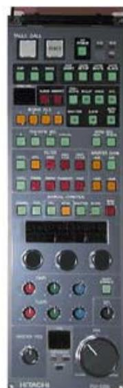
**SU-3300A:** Master Setup Control unit. Can directly access full setup parameters for 12 cameras and up to 48 with external delegation switch.
